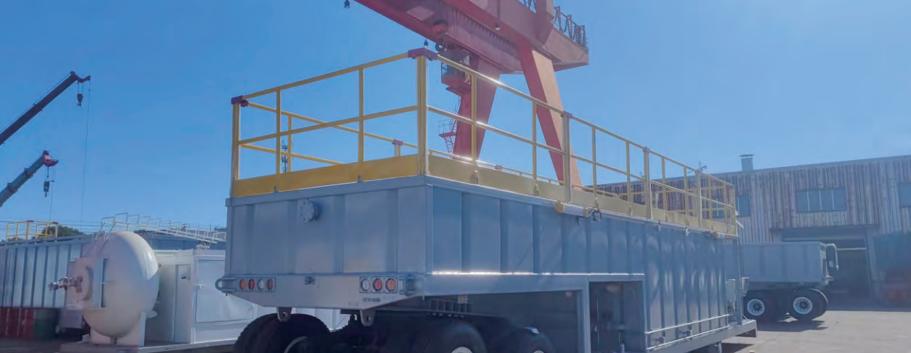
Trailer mounted fracturing liquid tank
